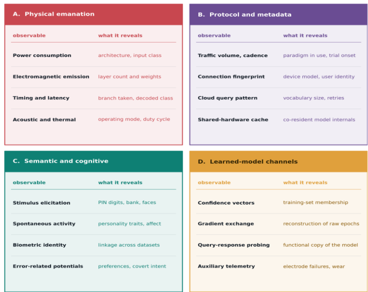
Figure 7. Four-family taxonomy of side-channel leakage in neural systems.
