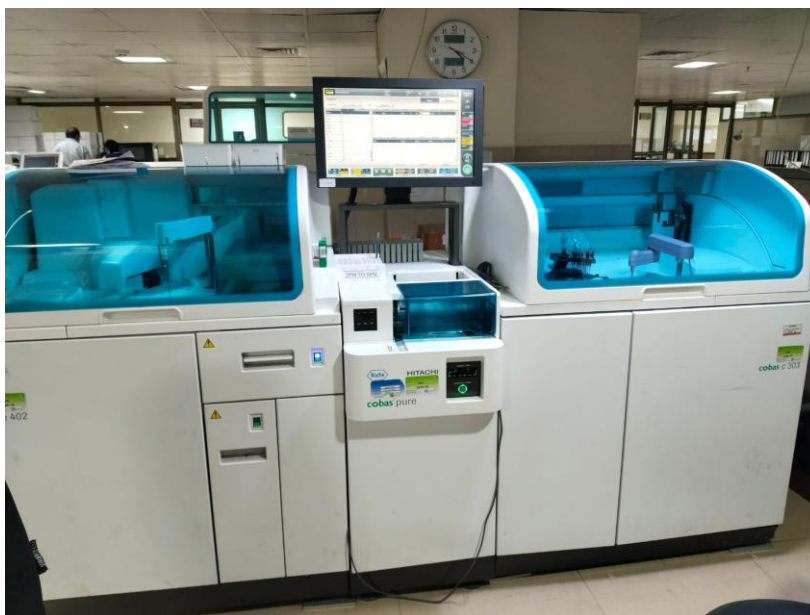
Figure 1. The COBAS Pure 6 Analyzer: A small laboratory device developed by Roche Diagnostics to provide very accurate results in clinical chemistry and electrolyte analysis. It includes automatic workflow systems for the efficient execution of various diagnostic tests.
