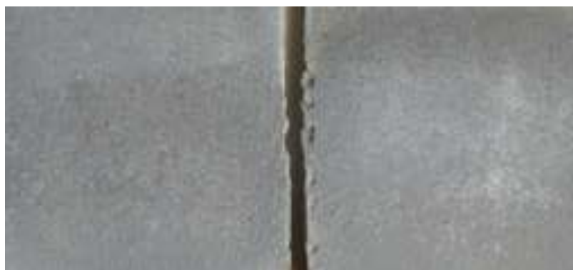
Figure 5:- Surface morphology of failure in Araldite® 2015 adhesive under tensile conditions.
