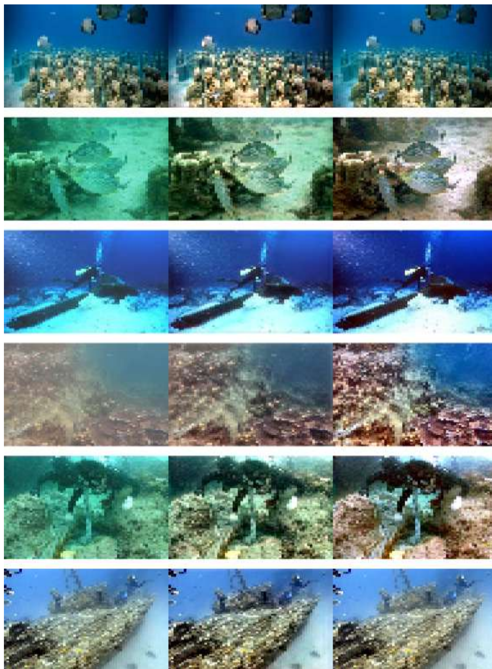
Figure 5: Raw input (left) / AquaRestore-UC output (centre) / reference (right) for six fixed-index test images from the completed seed-42 study (64×64, nearest-neighbour 4× upscaled for display). Rows top to bottom: 278_img_.png, 433_img_.png, 449_img_.png, 232_img_.png, 443_img_.png, 705_img_.png. The first and last rows are two of the twelve images in Table 6 where AquaRestore-UC reduces PSNR relative to raw input.
