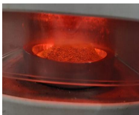
Figure 6. Determination of moisture content by drying the sample at 105°C.
