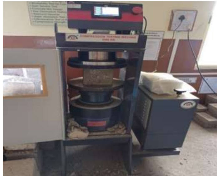
Fig.14 Testing of Compressive Strength using 2000KN compression testing Machine
