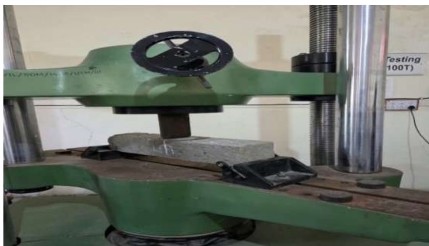
Fig. 15 Sample test of Flexural Strength test using UTM
