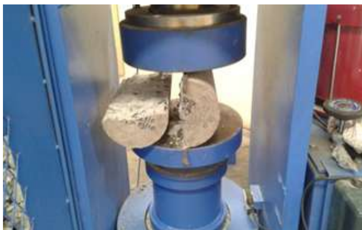
Fig. 17 Sample test on Split tensile test apparatus
