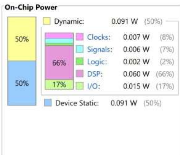
Figure 12 Power analysis of EMI filter on Artix 7
