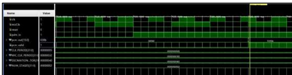
Figure 9 Simulation waveform of audio model of assistive device on FPGA
