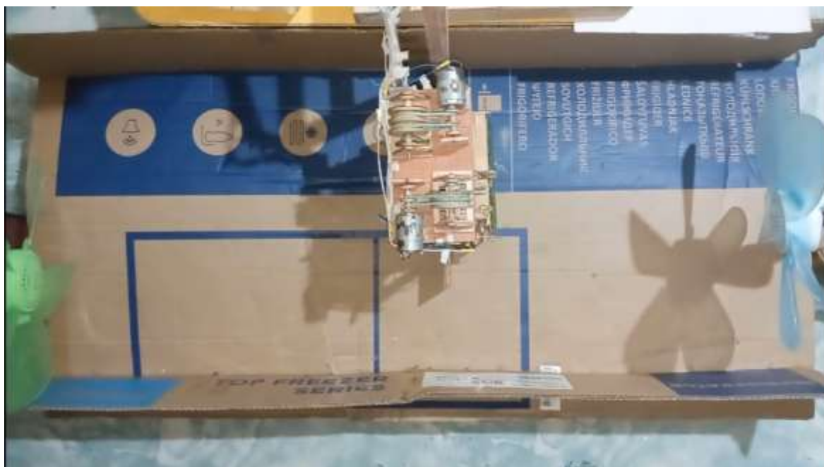
Figure 3 Controlled airflow arrangement with the prototype, simulated bank, and opposing electric fans.
