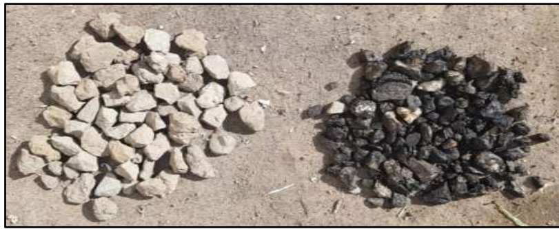
Figure 3. Uncoated and Coated aggregate for Binder Course
