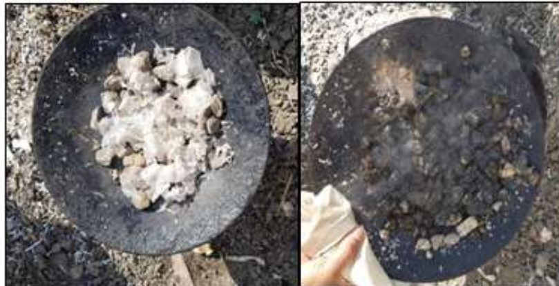
Figure 2. Plastics mixing with aggregates
