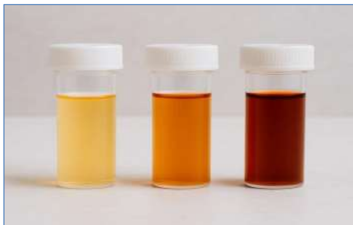
Figure (2) The solutions samples of natural Capsanthin dyes of at different concentrations
