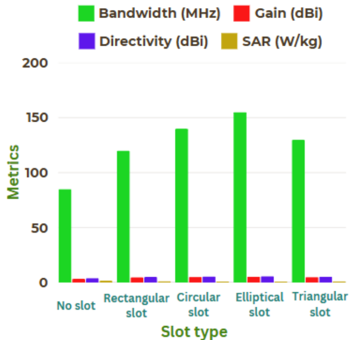
Figure.3. The effect of slot-loading on antenna performance
