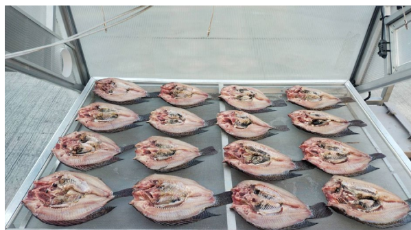
Fig 7. Experimental setup and distribution of prepared Nile Tilapia specimens on the PGSD drying tray
