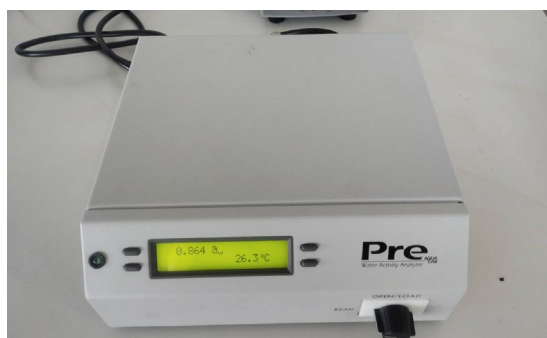
Fig 6. Water activity meter (AQUALAB PRE, USA)
